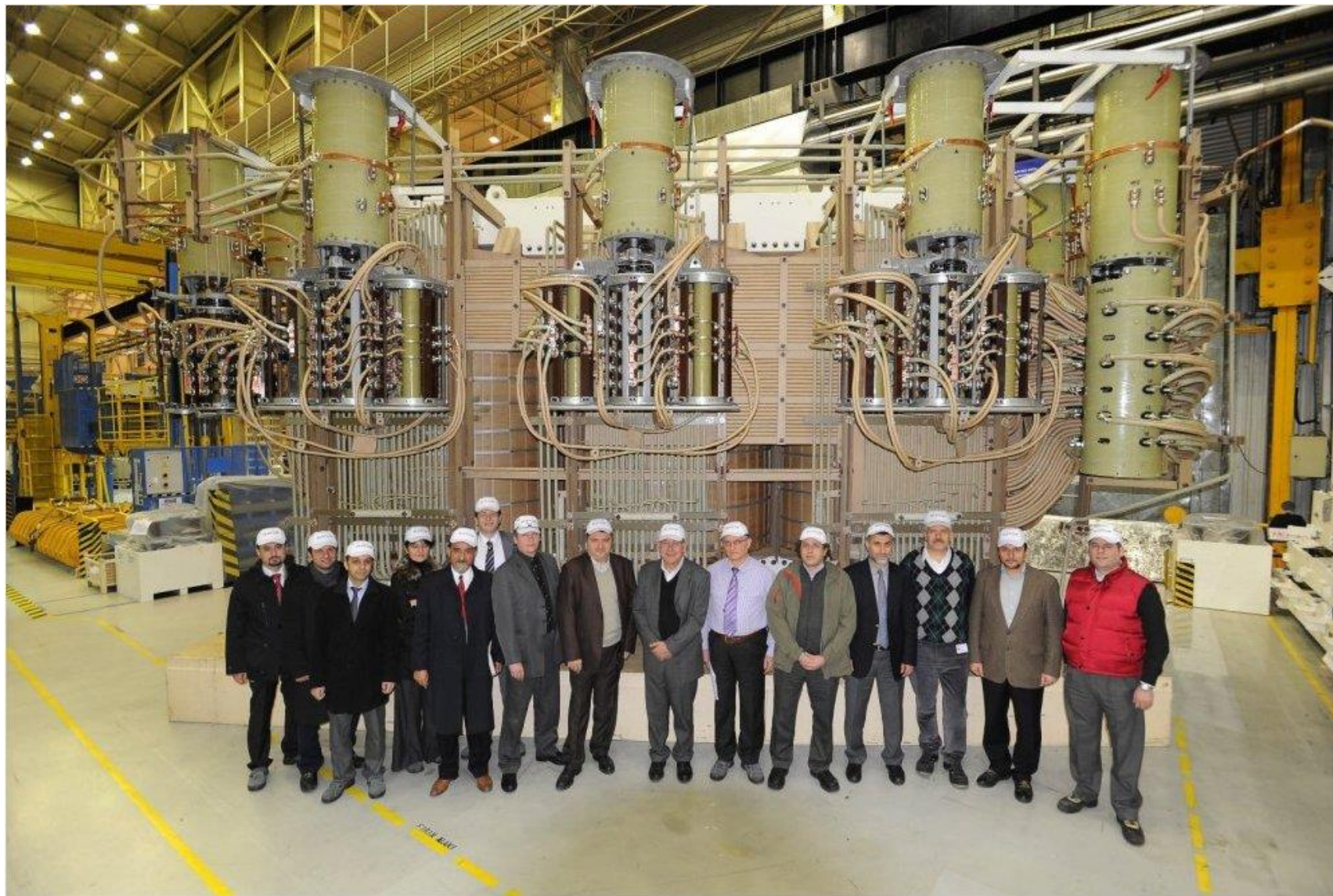
575-MVA phase-shifting transformer from Consolidated Edison for New York City with MR OLTCs
